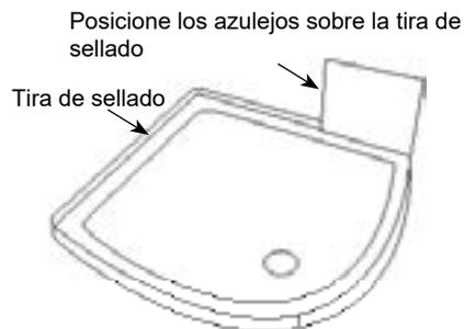
Install the shower tray in the correct position and tile in front of the seal strip.
